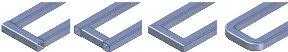
opposite, with the shortest member being trimmed against. You can mix and match frame component sizes and shapes and their end condition treatments; any combination is possible.
