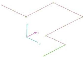
In addition to creating path segments from 2D sketches, you can also use edges and other geometry from 3D parts in the assembly. You also can build frames that have more than two frame members joined at a single vertex, choosing which of several possible solutions you want to use for mitering or cutting each of the frame members.
