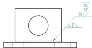
**Stitch weld** Where strength or gas tightness is not a priority, stitch welds are used to save time and materials. The Stitch Weld command provides a dedicated tool to apply stitch welds to join components. Options allow you to control the stitch length, gap size, style and offset values for perfect control.
