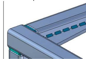
**Mirror and patterning** To help speed up the weldment process, weldments can be patterned or mirrored to other areas of the weldment.
