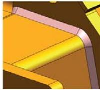
**Customized welds** Not all welds are simply triangular in shape; some beads need to represent a specific cross-section, either because of the weld specification or preparation type. Assembly feature tools – protrusion, revolved and sweep protrusions – are available so that users can define their required weld bead cross-section.
