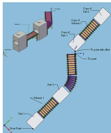
designs, a new manual component positioning capability allows existing subassemblies to be quickly copied, moved, rotated or arrayed within an assembly. To remove any restrictions, assembly relationships to existing components are ignored, while
