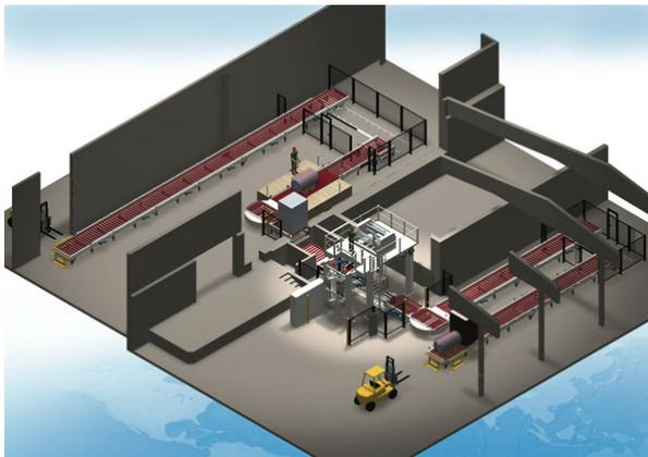
Often, simple 3D models of the machines are used to give a better sense of what the operation will look like. High quality renderings of a “completed” factory can enhance the overall presentation during the design review phase. With some simplified 3D models, fly-through animations are often used to show how people will work and how vehicles can move around the floor.
