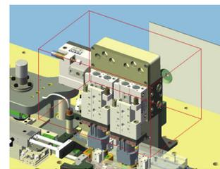
**3D box select** provides quick graphical selection of components being displayed.
