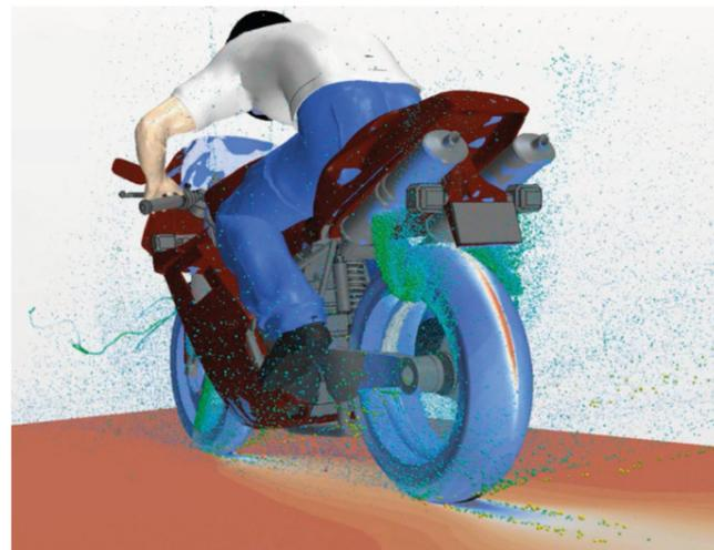
Lagrangian multiphase and fluid film interaction for water management of a motorcycle
