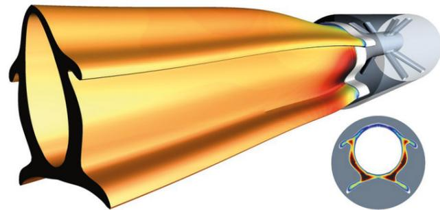
Rubber seal extrusion from a die
