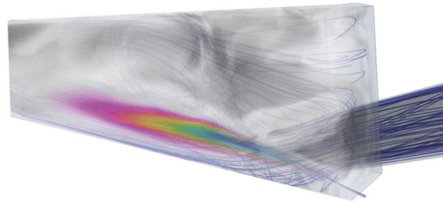
Mass fraction of CO in a glass furnace simulation
