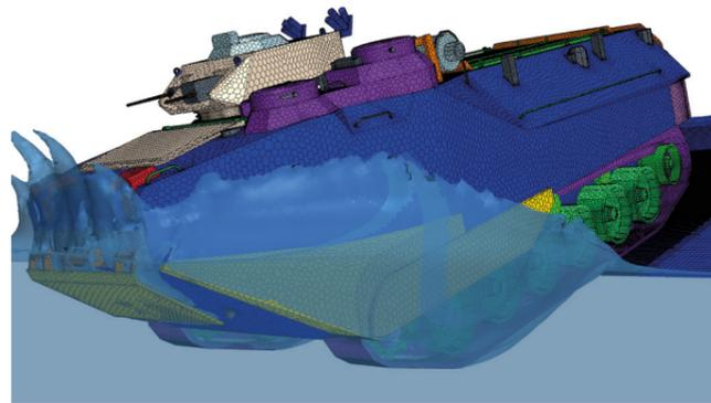
Water entry analysis of an Assault Amphibious Vehicle (AAV7) with Overset Mesh
