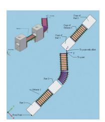
semblies to be quickly copied, moved, rotated or arrayed within an assembly. To remove any restrictions, assembly relationships to existing components are ignored, while those integral to the subassembly remain intact. Subassemblies can be simply dragged to a new location or precisely moved using coordinates, vectors or exiting components.
