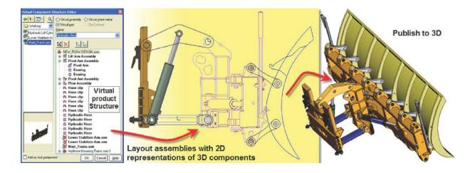
Once 3D data is imported into Solid Edge, powerful tools add additional intelligence and allow quick and easy editing. Auto Constrain adds parametric relationships to imported assembly files. OEM supply chains are able to assemble their designs in Solid
