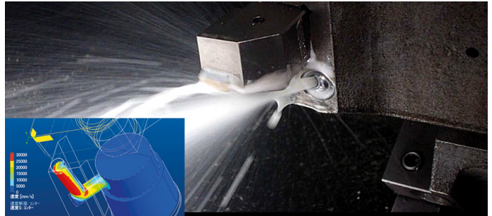
Mitsubishi materials corporation uses Simcenter FLOEFD to design liquid-cooled nozzles for cutting tools
