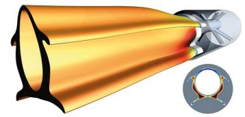
Rubber seal extrusion from a die
