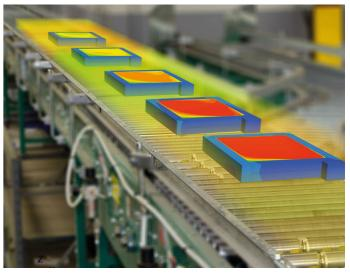
Evaporator exiting from brazing furnace (Courtesy: Denso Subros Thermal Engineering Center, India)
