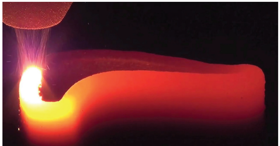
3D printing with a metal deposition nozzle.
