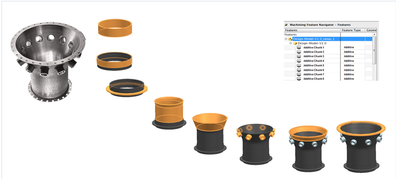
Automatic and semiautomatic decomposition of parts into features for additive/subtractive operations definition.
