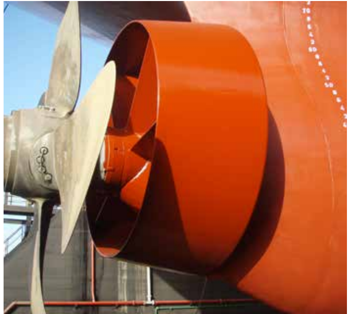
IBMV utilized a STAR-CCM+ digital twin to design the Becker Mewis duct in six weeks, delivering $500k per year per ship in fuel savings
