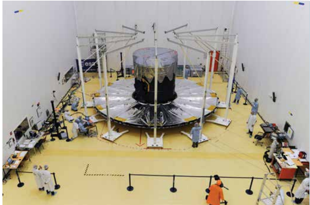
Gaia Deployable Sunshield Assembly (DSA) integrated onto the spacecraft and undergoing deployment testing in Toulouse.
