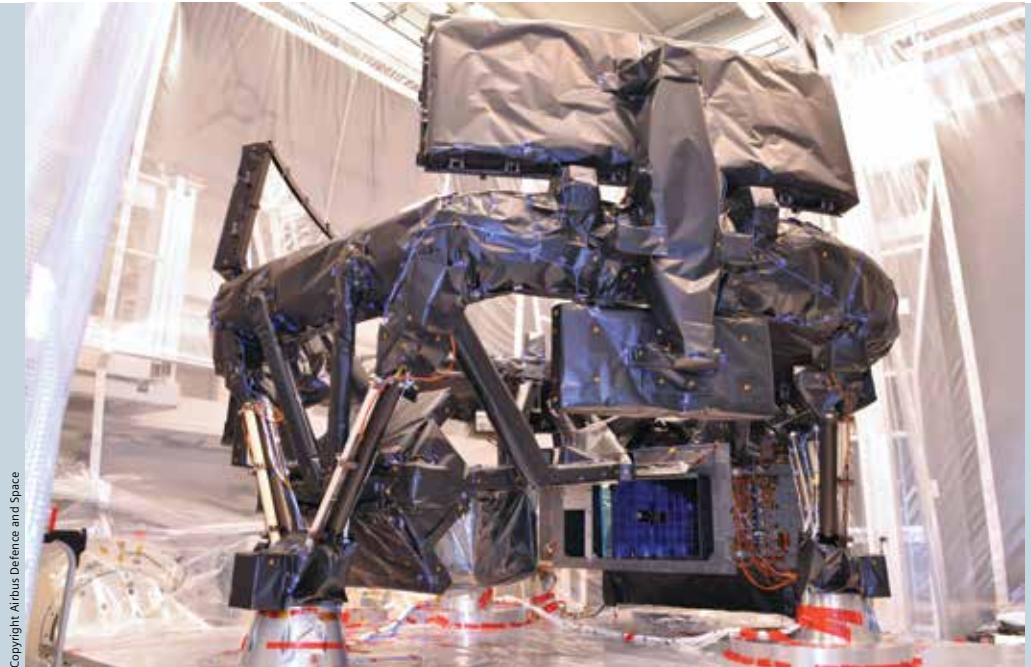
The Gaia payload module instrumented for environmental testing at the test center of Airbus Defence and Space in Toulouse, France.
