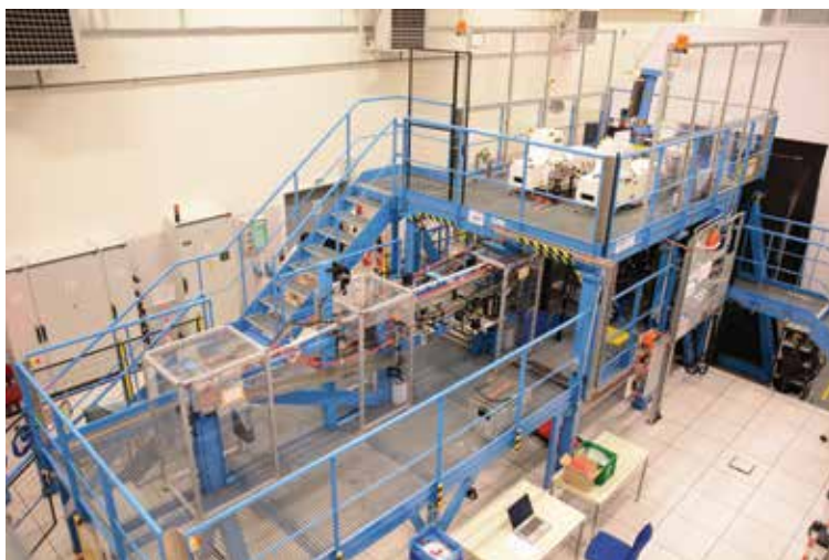
The virtual iron bird of the Airbus H160 at the test facilities of Airbus Helicopters Research and Development in Marignane, France.
