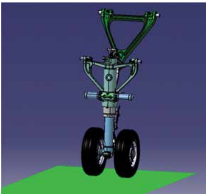
Parameterized landing gear simulation model established using Simcenter 3D.
