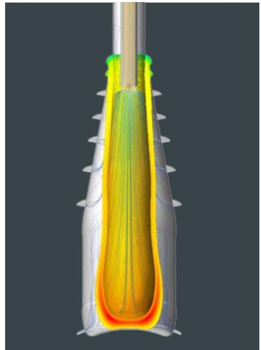
*“We have very complex physics. The structural and fluid dynamics aspect of the cooling of molten glass cannot be separated because they are very, very, coupled. Understanding the actual temperature of the glass is by far the most important factor in ensuring the strength and quality of the final container. Multiphysics simulation using a tool like STAR-CCM+ is the only way that we can achieve that.”*
