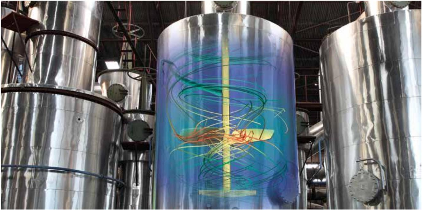
STAR-CCM+ brings automated design exploration and optimization within the grasp of all simulation engineers. Shown here is a mixer design study starting with a baseline (left) and resulting in an improved design (right) with a fourfold decrease in power consumption while maintaining blend time. The final prototype is pictured above.
