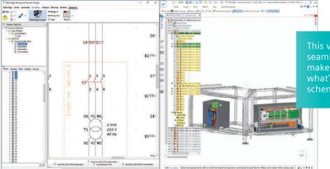
This view of the wiring in a seamless MCAD-ECAD environment makes it easier to understand what's portrayed in an electrical schematic.
