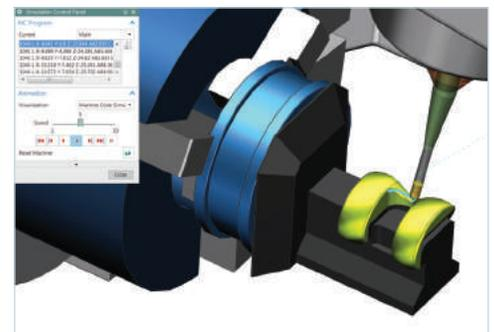
account of any program content provided by the postprocessor. Home positions, special tool change motion and other content can be inserted by the postprocessor, minimizing surprises by making sure to simulate the posted g-code.
