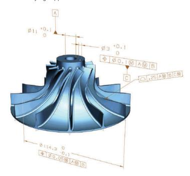
Automate creation of inspection programs by using PMI on CAD model.
