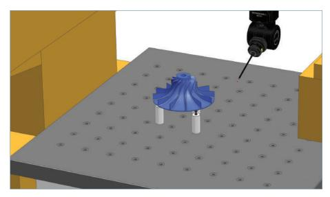
Leverage the machine environment to easily design holding fixtures.
