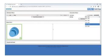
The web-based platform searches not only Solid Edge parts, but also parts authored in other computer-aided design (CAD) software. Smart thumbnail images provide visual feedback, while a wide range of property filters and similar adjustable settings allow users to sort parts.
